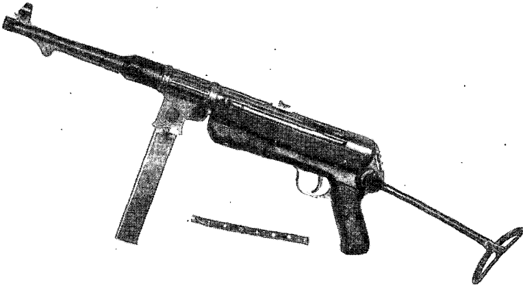
Figure 39.—9-mm submachine gun ( Schmeisser M.P. 38 ) with magazine attached and shoulder rest extended.
